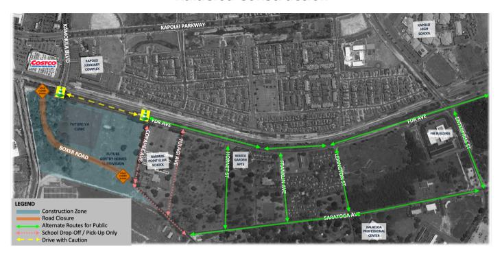
**FDR Ave:** Changes from 2-lanes to 4-lanes along the entire length of the project with two lanes in each direction. This new segment will have sidewalks on both sides of the road, which will increase walkability in the area.
